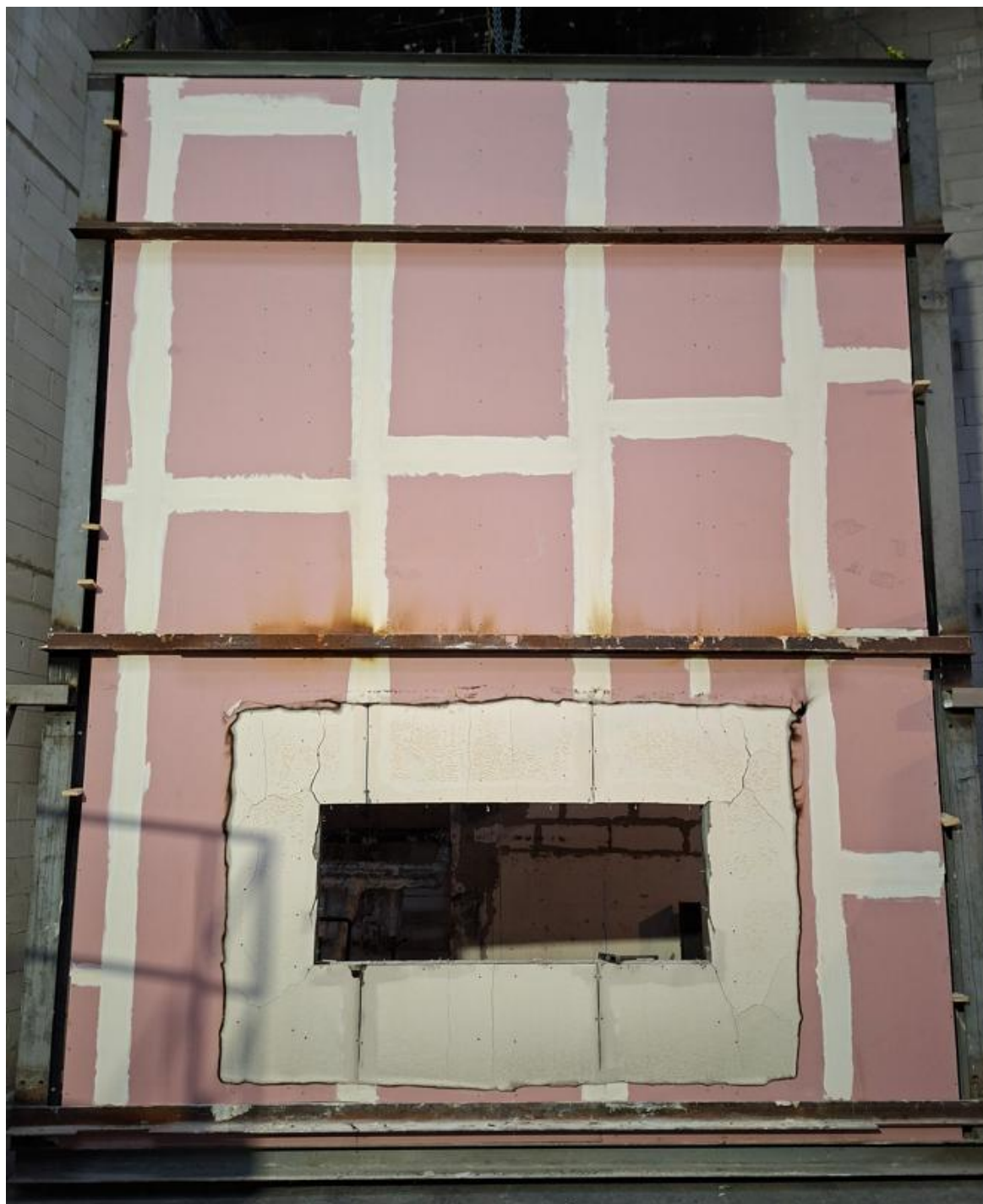
Back part of the base wall It is noticed that the flame didn't spread to the second storey room
