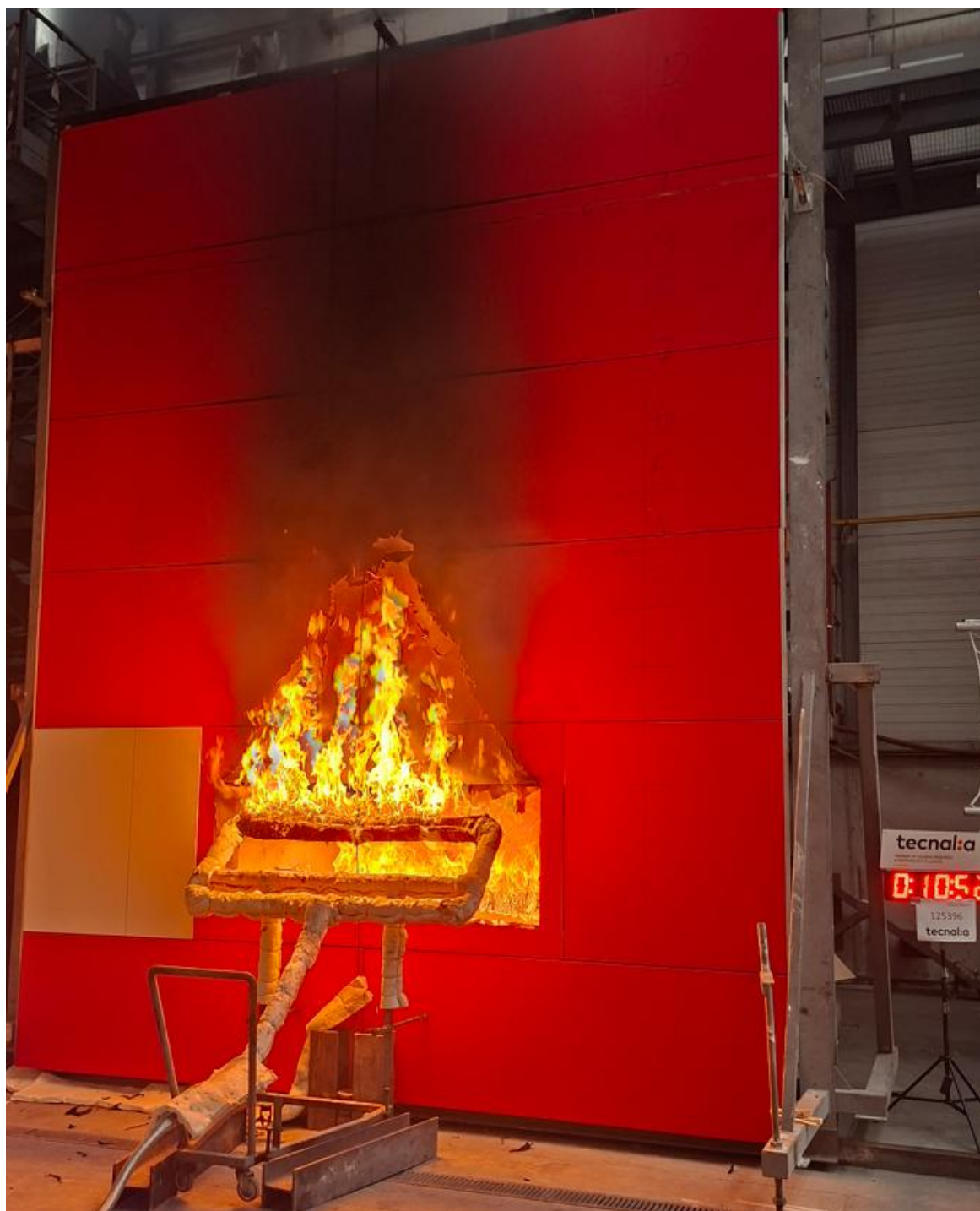
General view of façade system test specimen during testing
