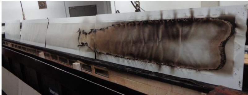
Photo No. 5 Exposed Surface of the Test Specimen (Post-test)
