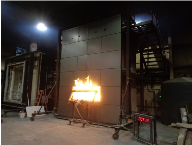
Photo No. 8 Window Burner Ignition
