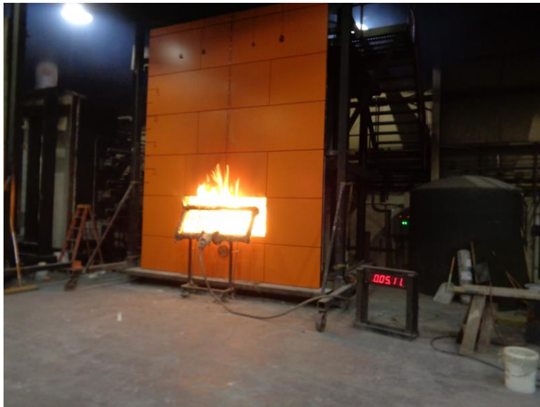
Photo No. 8 Window Burner Ignition
