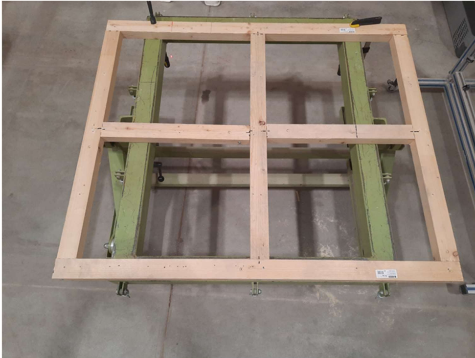
Pic. 1 Substructure Wooden bar 60/40 mm
