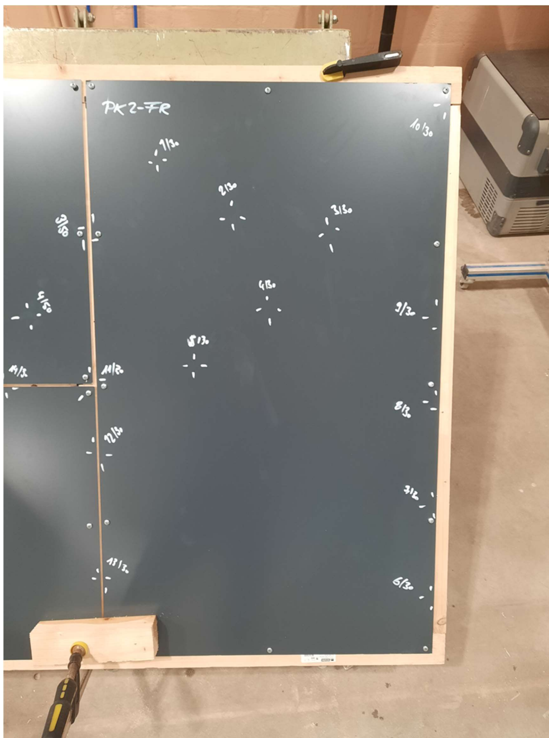
Pic. 4 None visible dents after shooting with 3 cm IB
